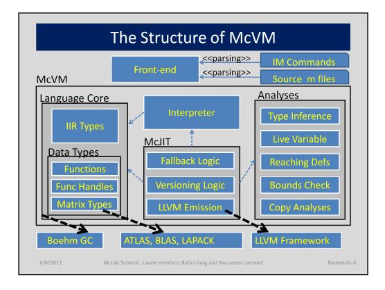
The front-end is responsible for parsing matlab commands and m files. The language core is supported by Boehm GC, ensuring an automatic garbage collection of IIR nodes. The operations on Matrix–type data are supported by ATLAS, BLAS and LAPACK library. McJIT is supported for efficient code compilation by several analyses.
