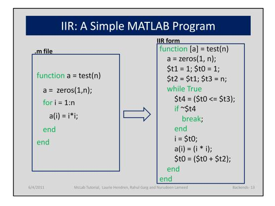
The box on the left-hand side shows the code of an .m file. This is transformed into the box on the right : the corresponding function in internal IR form.
