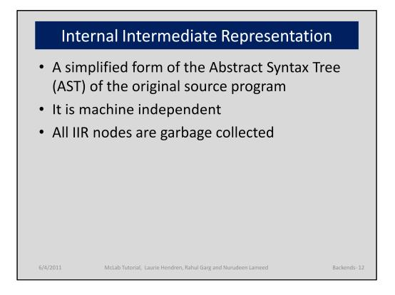
McVM converts source code into a form more amenable to analyses. It is similar in form to a three address code.
