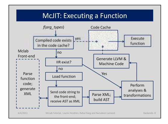
How does the JIT compiler execute a function? Given a function called with some argument types; McVM checks if a compiled code exists that match the call, in terms of the types of the arguments and proceed as shown.
