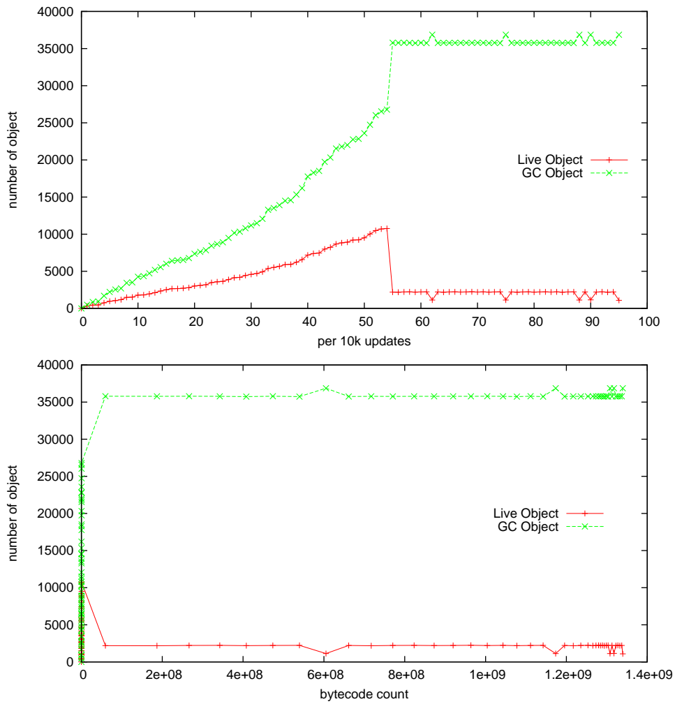
Figure 12: Power GC result for every 1k updates. At the top the time axis is in terms of total data structure updates, and at the bottom in terms of bytecodes executed.
