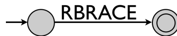
Figure 7.7 A high-level view of the reverse \epsilon -NFA generated for a single meta-pattern.
