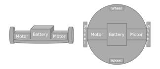
Figure 2: Overview of the Automated Guided Vehicle example.
